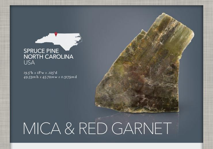
Sheets of mica are nothing if not versatile. From prehistoric times up to today, they've been used for everything from simple windows and ancient accessories to modern electronics and atomic-force microscope components.
